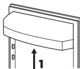
To permit storage of food packages of various sizes, the door balconies can be placed at different heights.
